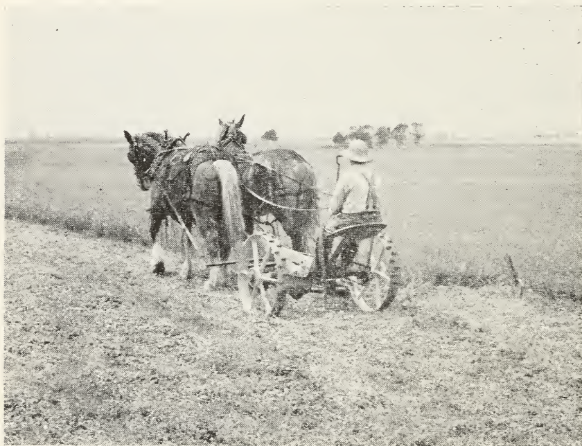
FIGURE 2.—Horse-drawn mowers are used by many farmers who have small acreages of hay to harvest, and who use the lesser mechanized methods of harvesting. One 5-foot mower pulled by a good team will cut about 1 acre of hay in an hour.
